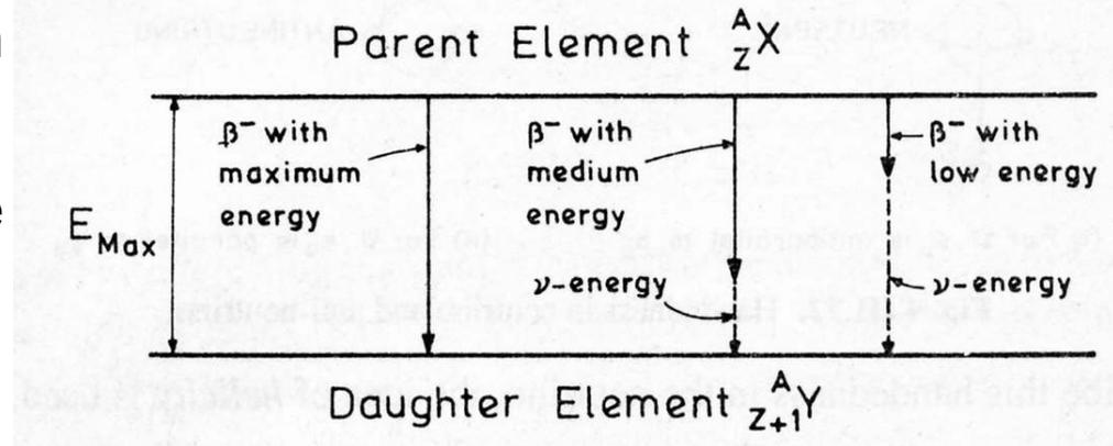
Diagram showing the sharing of total disintegration energy between the beta particle and the neutrino
